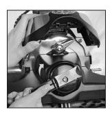
12 Use the handle on the Multi-Surface Shampoo Nozzle Belt Lifter to turn it clockwise until the green arrows line up. Lower the Headlight Hood.
