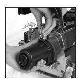
Remove the Power Nozzle. See Page 22. Place the hooks on the back of the Air Intake Guard over the Attaching Bar on the front of the unit. Push the Air Intake Guard up against the unit and turn the Accessory Lock clockwise to secure.
