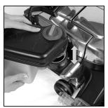
2 Attach the empty Shampoo Tank to the Air Exhaust Port. It is not necessary to attach the elbow hose. This setting allows airflow through the system.
