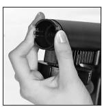
3 Press the two latches on the front of the nozzle jet, pull it out, and thoroughly rinse. Fill the jar with water, reattach and spray water until clear.
