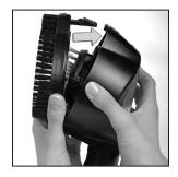
3 Place the turbine back in the tool and turn it until the tabs drop into the slots. Snap the brush ring back into place.
