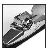
5 Flip out the handle on the Belt Lifter on the Power Nozzle. Turn it counterclockwise until the red arrows line up. The hook should catch and stretch the Belt inside the Power Nozzle.
