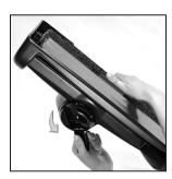
While pushing up on the belt with your finger, use the handle on the Belt Lifter to turn it counterclockwise until the red arrows line up. The Belt Lifter Hook will catch and stretch the belt.
