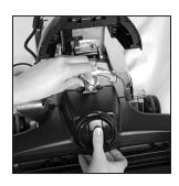
11 Push the Multi-Surface Shampoo System up against the unit and turn the Accessory Lock clockwise to lock in place.
