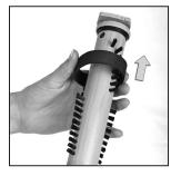
$oldsymbol{\Lambda}$  Slide off the old belt and replace with a new one.
