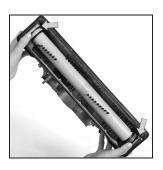
3 Note the bristle height setting which is marked on the end of the Brush Roll before lifting out the Brush Roll. See page 55.
