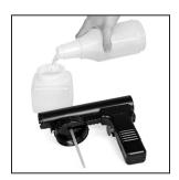
1 Set up the Portable Sprayer. Unscrew the jar and fill it 3/4 full with non-flammable liquid.
